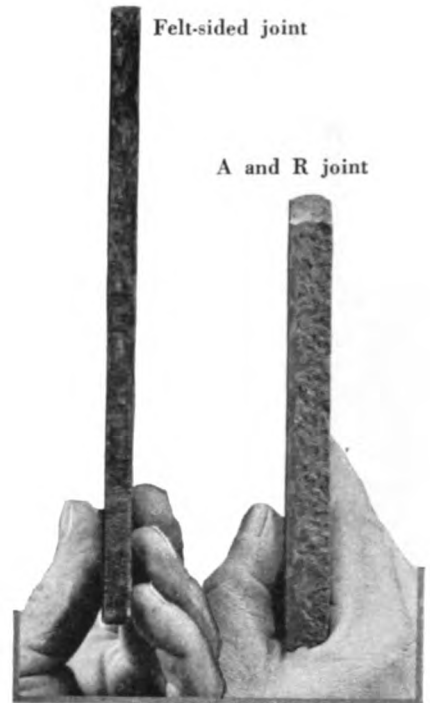
The A and R joint returned to its original thickness, while the felt-sided joint was permanently deformed
