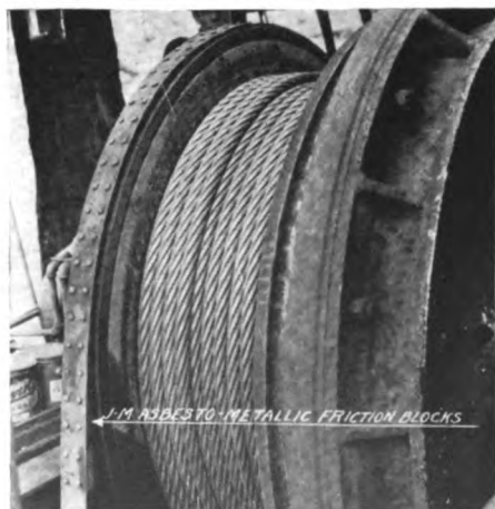
Only one set of J-M Asbesto-Metallic Brake Blocks on a brake that handled 53 million feet of lumber in 2 years
