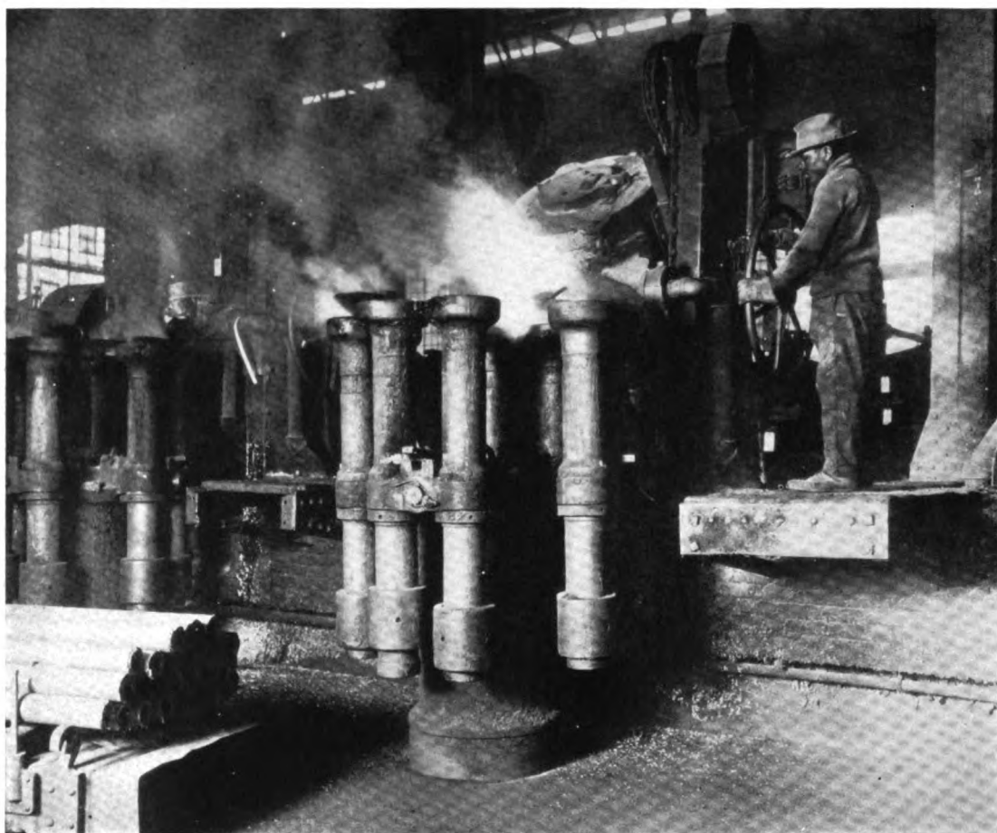
An Ajax-Wyatt electric induction furnace with a monolithic lining of No. 34 Refractory Cement
