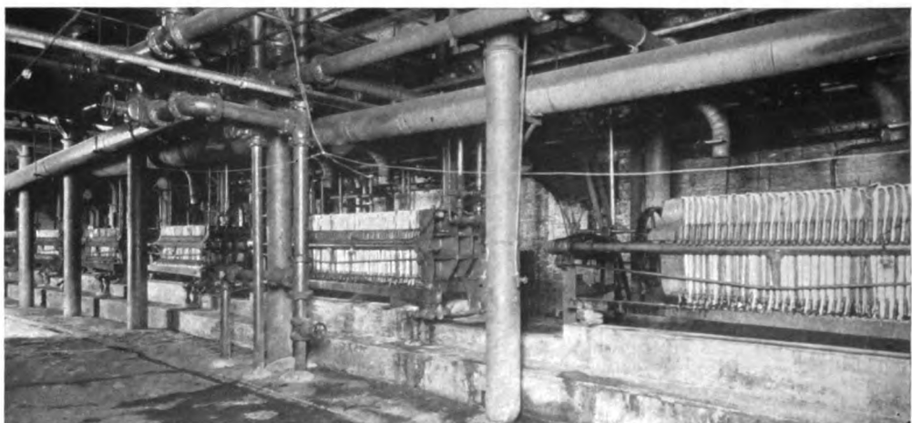
Fig. 6. Celite Filter-Aids are used in this battery of filter presses for the clarification of high-grade syrups.
