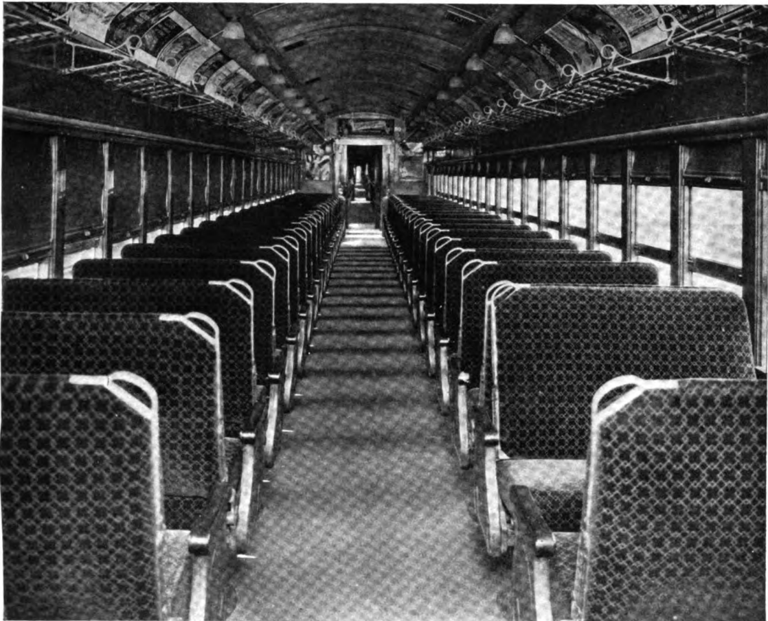
Suburban car on the Chicago & North Western Railway, floored with J-M Masticoke
