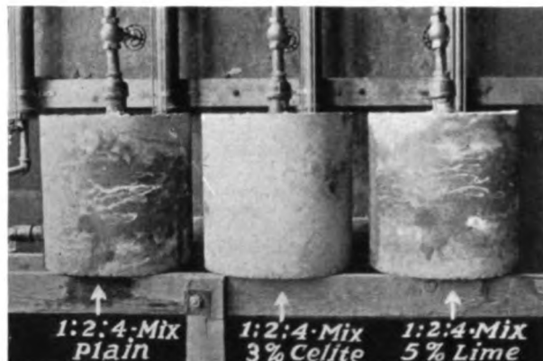
Fig. 10. Permeability test by Pierce Testing Laboratories, Inc., Denver, Colorado. Photographed after completion of test, maximum pressure 200 lb. per sq. in. Note relative dryness of Celite cylinder
