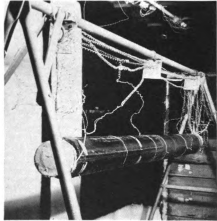
An interior view of the "cold room" in which insulations for service in the low temperature range are tested. The temperature in this room can be automatically regulated and kept constant down to zero degrees F.
