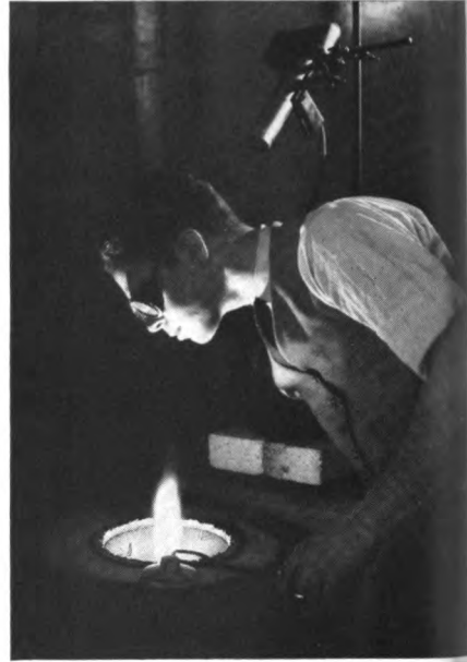
A scene from the Johns-Manville Research Laboratories where "Guardians of the B. t. u." are on constant vigil in their efforts to control heat. That is not flame coming from this Ajax-Northrup electric induction furnace. It is white heat. The furnace was at 3200° F. when the photo was taken.
