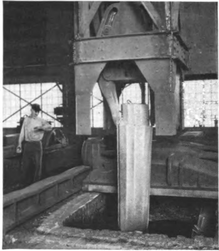
Stripping crane removing hot ingots from a soaking pit. This pit was insulated with 4 inches of Sil-O-Cel C-3 Concrete in the base and Superex Blocks and Sil-O-Cel Natural Brick in the walls and over the top.
