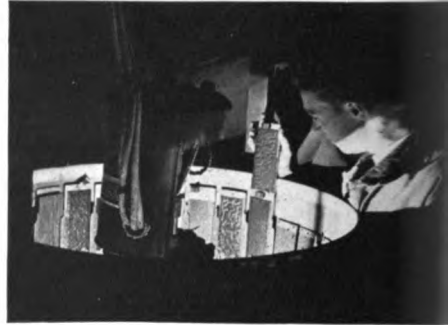
Inspecting samples of material in the Weatherometer, a machine in the Johns-Manville Research Laboratories which reproduces sunshine, rain, and freezing temperatures in cycles for the accelerated weathering of insulation jackets and casings in order to test their ability to withstand exposure to the elements.
