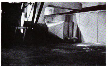
Dryer housing made of Transite-Encased Insulating Board
