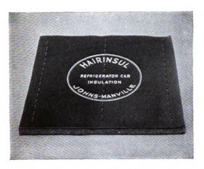
J-M Hairinsul refrigerator car insulation is a blanket type of insulation which consists of either all cattle hair or a mixture of cattle hair and other fibres in specified proportions, all chemically cleansed, felted between two layers of waterproof paper and stitched on approximate 5" centers.
