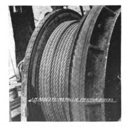
Only one set of J-M Asbesto-Metallic Brake Blocks on a brake that handled 53 million feet of lumber in 2 years
