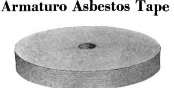
Armaturo Asbestos Tape is especially adapted to magnet and armature work. It is a combination of asbestos fibre and cotton mesh cloth, the asbestos fibre being run up on both sides of the cotton mesh without filler or sizing. The asbestos insures dielectric and heat-resisting qualities, while the cotton mesh gives strength, the latter being particularly desirable where the product is used in connection with winding machines.
