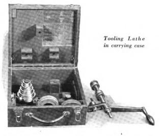
When using Harrington Joint Conduit, long radius bends may be satisfactorily made up with the tooling lathe by using short sections of Fibre Conduit joined with couplings. It is not recommended that this practice be followed on curves with less than a 5-ft. radius, as the conduit ends, under such conditions, may offer resistance to the rodding wires or cable grips. This plan is not recommended for Socket Joint Conduit, as the joints would not be sufficiently tight.
