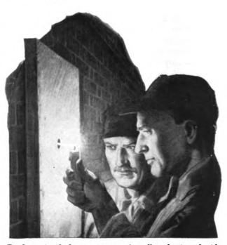
To determine leakage, a square of cardboard, pierced with a small hole and fastened to a wood frame, may be pressed against a boiler wall and the edges temporarily sealed. The inrush of air through the hole shows the leakage.
