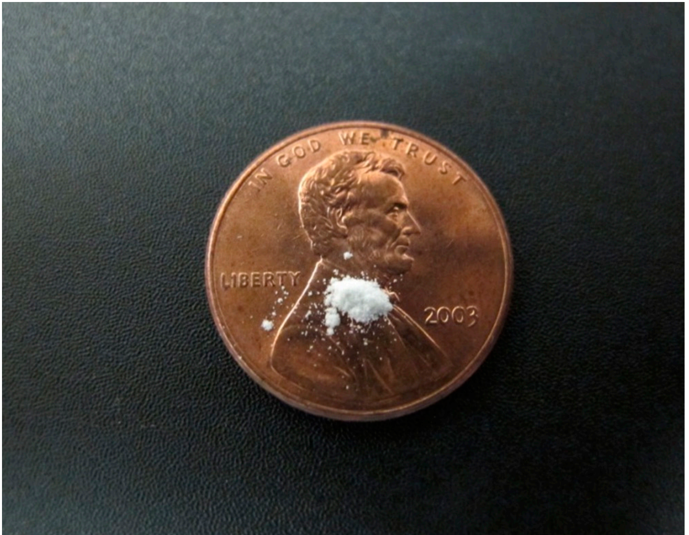
Figure 6. Ten milligrams of talc for scale on a U.S. penny [24]. An equivalent amount of the Kelwa Marble Dust, as tested, would contain approximately 37,000 countable fibrous structures of the regulated asbestos mineral tremolite. Source: Authors [24]. U.S.: United States.
